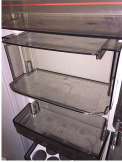
Missing front flap to one door shelf
